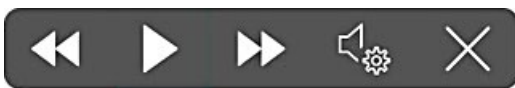
Figure 6. Microsoft Word’s Read Aloud function button controls. From left to right, they are Back, Play/Pause, Forward, Settings, and Exit.
